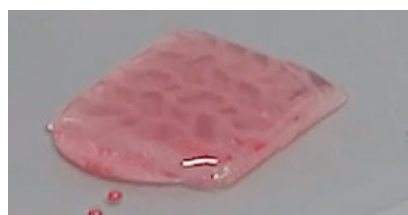
Printing at physiological conditions and submersion of the bioprint model in culture medium promotes cell survival and enables immediate handling of the scaffold.
