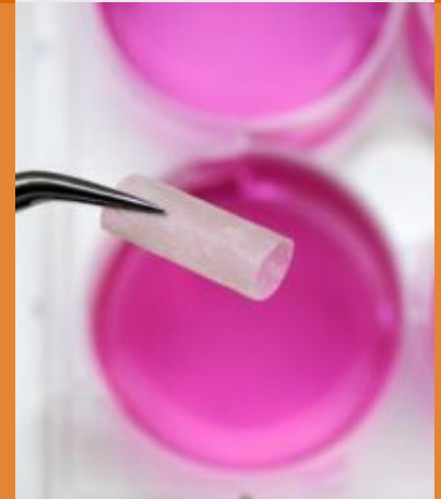
Collagen Bio Tubes for cell growth at in- or outside of the tube wall
